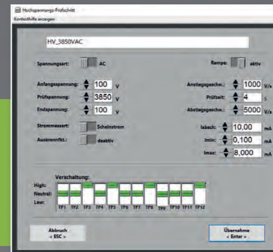
High-voltage test plan with switching matrix
