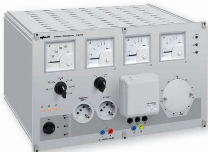
Example: tele-controllable three-phase supply
